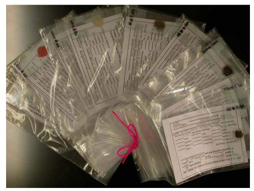
Figure 30. Samples prepared in microscope well-slides submitted to James Martin of Orion Analytical for FTIR and SEM-XEDS analysis.
