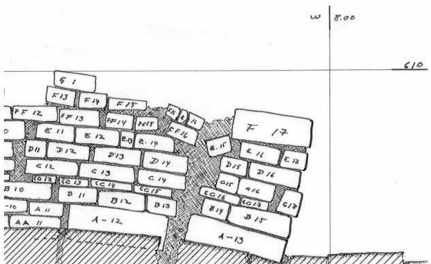
Figure 2. Example of adequate way to mark stones in preparation for anastylosis. Marks on the main face of stones are to be avoided.
